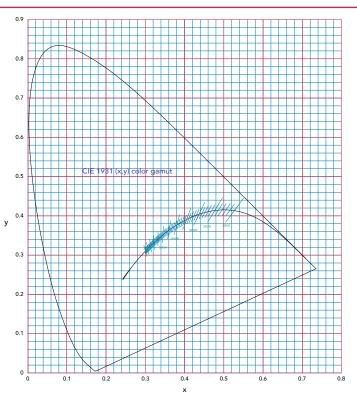
Figure 2: CIE 1931 (x, y) color space with the Black Body Locus (BBL) shown as a heavy black line. "Perfect" white light is exactly on the BBL. Major (green) and minor lines (blue) represent increments of 500 CCT and 100 CCT, respectively.
